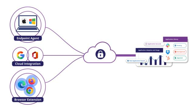
The Auvik SaaS Management **endpoint collector** is a Windows and macOS collector installed on each managed workstation in the environment. All configuration and data collected by the Auvik SaaS Management software on the workstation is encrypted on the disk. Data transmitted from the endpoint collector to the cloud is encrypted with SSL/TLSv1.2. The endpoint collector has four primary functions:
